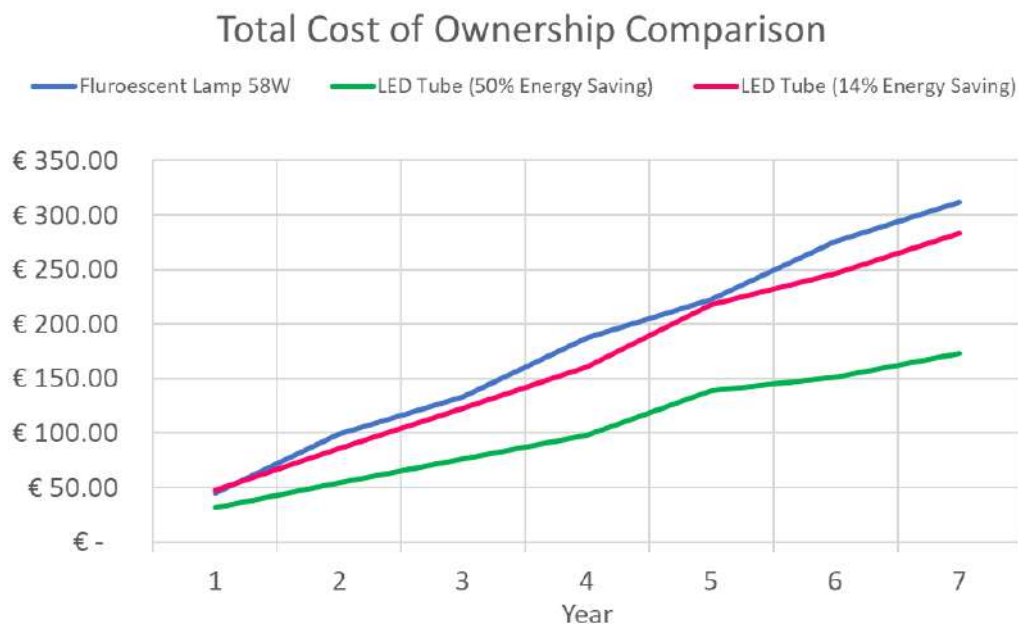
Figure 5. Chart showing the potential disruption in the total cost of ownership if an LED installation involves electronic ballasts that draw much higher power, compared to the LED lamp's rated value.
